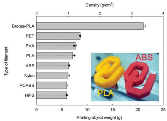
**Figure 2.** Average weight of printed object for each filament (horizontal bar) with standard deviations (error bar) and known material densities (black dot).
