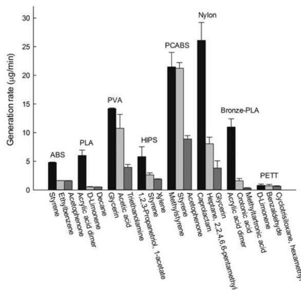
**Figure 8.** Generation rate ( $\mu\text{g}/\text{min}$ ) with standard deviations (error bar) of top three VOC markers for each filament.
