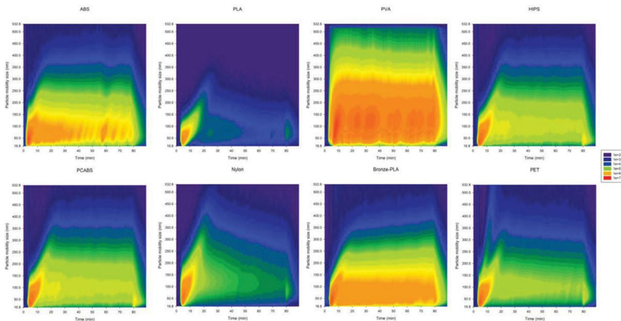
**Figure 4.** Evolution of particle (mobility) size distribution based on number concentration in the sub-half-micron size range (16.8–532.8 nm) as a function of time (min) for each filament.
