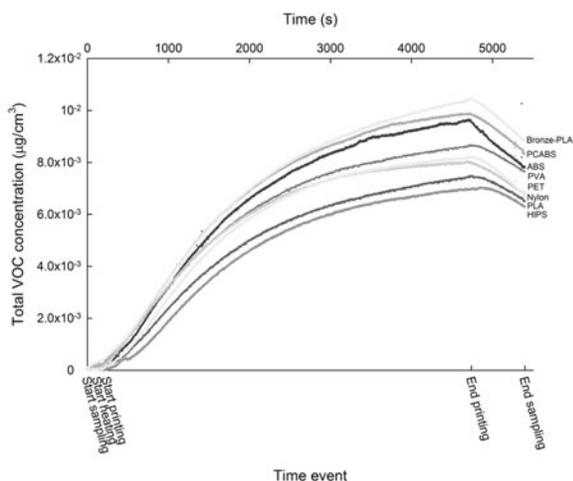
**Figure 7.** Total VOC concentration ( $\mu\text{g}/\text{cm}^3$ ) in the chamber measured by photoionization sensor.
