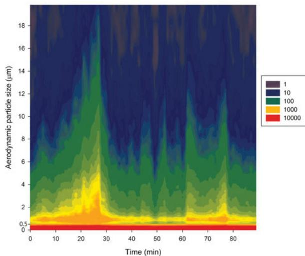
**Figure 5.** Average evolution of particle (aerodynamic) size distribution based on number concentration in the super-half-micron size range (0.5– $20\ \mu\text{m}$ ) as a function of time (min).
