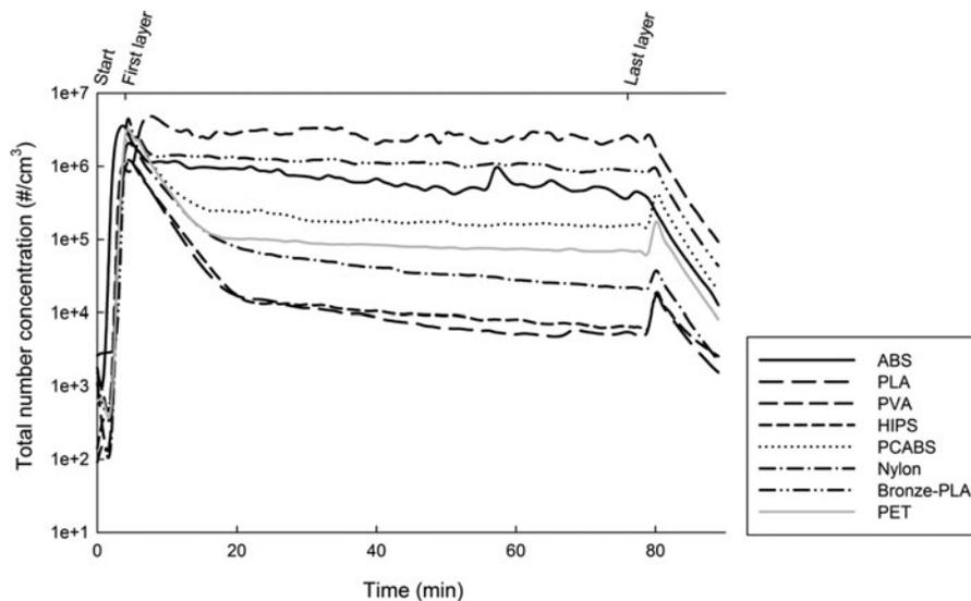
**Figure 3.** Particle number concentration ( $\#/cm^3$ ) in the sub-half-micron size range (16.8–532.8 nm) as a function of time (min) for each filament.
