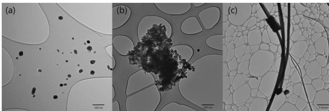
**Figure 6.** TEM images of fume particles on scales of: (a) 100 nm, (b) 250 nm, and (c) 2  $\mu\text{m}$ .
