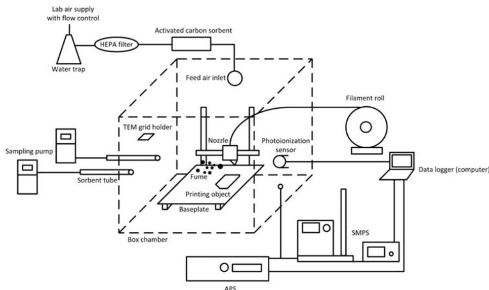
**Figure 1.** Schematic diagram of the testing chamber.
