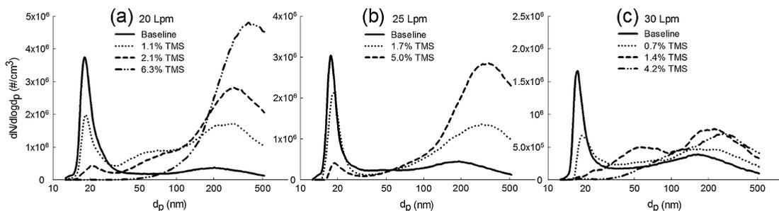
**Fig. 4.** GMAW fume particle size distributions at (a) 20, (b) 25, and (c) 30 lpm shielding gas flow rate. Note: total particle number concentration decreased as shielding gas flow rate increased.
