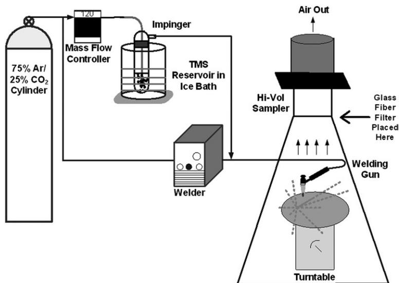
Fig. 1. GMAW fume generation and sampling system.
