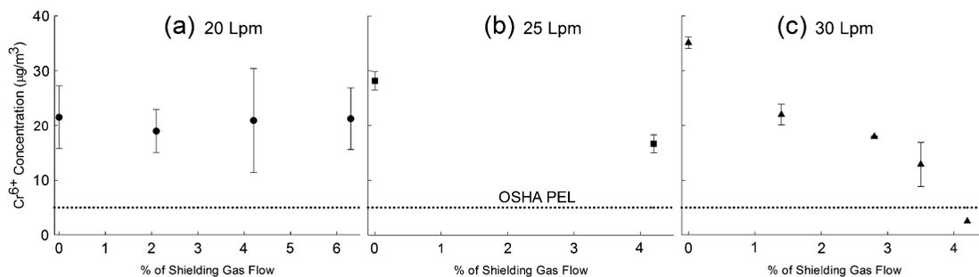
**Fig. 2.** Average Cr<sup>6+</sup> mass concentration as a function of TMS carrier gas flow rate at (a) 20, (b) 25, and (c) 30 lpm total shielding gas flow rate. Baseline samples using no TMS are presented closest to the y-axis in each figure. The values on the x-axis denote how much of the total shielding gas flow rate is used as TMS carrier gas. The data point to the far right of (c) has no error bar because all samples were below the detection limit.
