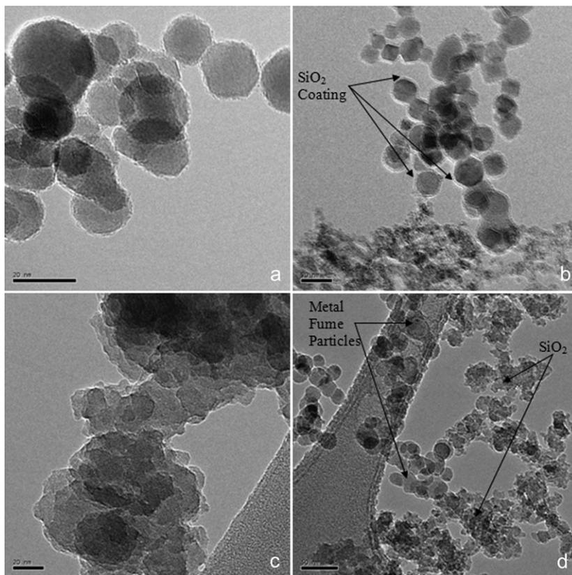
**Fig. 5.** TEM images of welding fume particles collected at 4.2% of TMS carrier gas flow rate with 30 lpm of total shielding gas flow rate: (a) GMAW fume agglomerate without  $\text{SiO}_2$  coating (scale = 20 nm); (b) GMAW fume agglomerate with  $\text{SiO}_2$  coating indicated by arrows (scale = 20 nm); (c) amorphous  $\text{SiO}_2$  agglomerate (scale = 20 nm); (d) metal- $\text{SiO}_2$  agglomerate formed by intercoagulation (scale = 50 nm).
