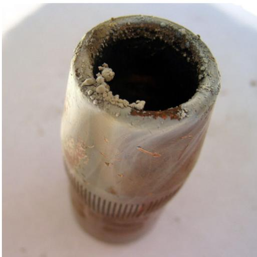
**Fig. 3.** Head of the welding torch gas nozzle (inner diameter = 0.97 cm) after sampling showing white powder from premature decomposition of TMS using 20 lpm of welding shielding gas.
