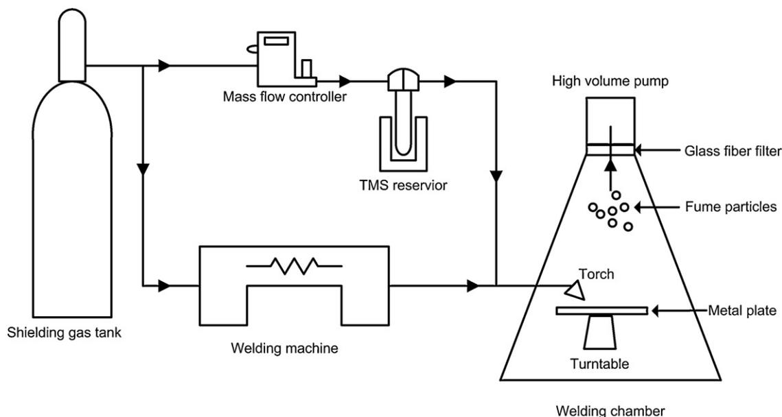
Fig. 1. Schematic diagram for the sampling system.
